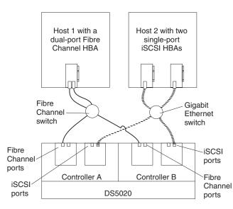
Figure 63. Example of iSCSI and Fibre Channel hosts, multiple-port configuration
